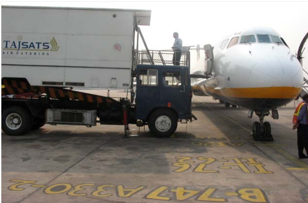
The Catering Hi-Lift was aligned & catering carried out
